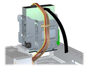
5. If removing an optical drive, disconnect the power cable (1) and data cable (2) from the rear of the optical drive.
